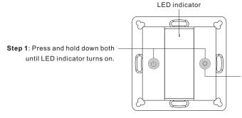
Step 2: Short press 5 times continuously to clear all bound lighting devices. LED indicator flashes 4 times for successful unbinding.
